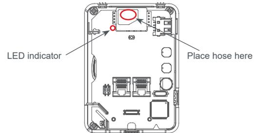
\*Note that the CO<sub>2</sub> sensor has an optical bench that flashes. This is not the LED. The LED is at position D6 on the board. See diagram above.
