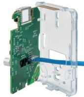
6. Swing the circuit board closed, ensuring the RJ-45 cables are tucked sufficiently into the wall opening to allow for complete closure using the locking tab.
