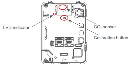
\*Note that the CO<sub>2</sub> sensor has an optical bench that flashes. This is not the LED. The LED is at position D6 on the board. See diagram above.
