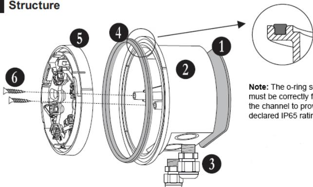
**Note:** The o-ring sealant must be correctly fitted in the channel to provide the declared IP65 rating!
