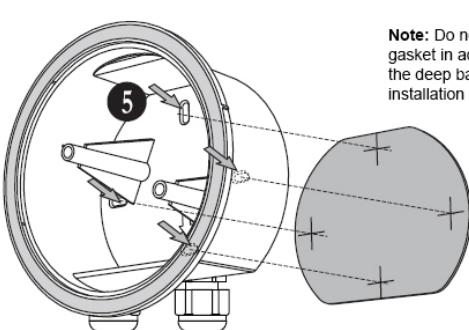
**Note:** Do not drill holes in the solid rubber gasket in advance! Place the gasket behind the deep base and fix them together to the installation surface.
