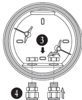
**Note:** Place the back box in upright position; Mount cable glands with IP65 into the holes and tighten the nuts underneath.
