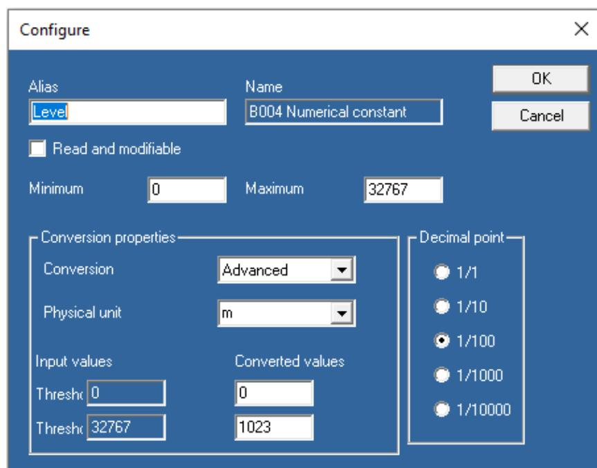
If the value of **Level** is 32,767, the communication interface converts it into meters. The value that will be sent in the alarm message will be 3.00 m.
