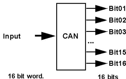
**NOTE:** This function can be used for example to break down a **Modbus**, page 183 type input (**J1XT1...J4XT1**) and to duplicate these statuses in the discrete outputs.
