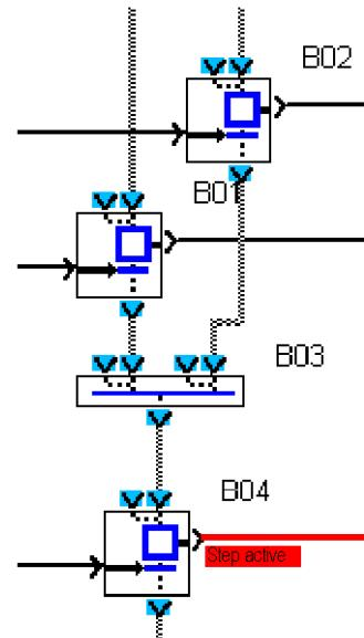
**Example 2:** transition 1 and transition 2 are made simultaneously passing while operating phases 1 and 2 are simultaneously in progress.
