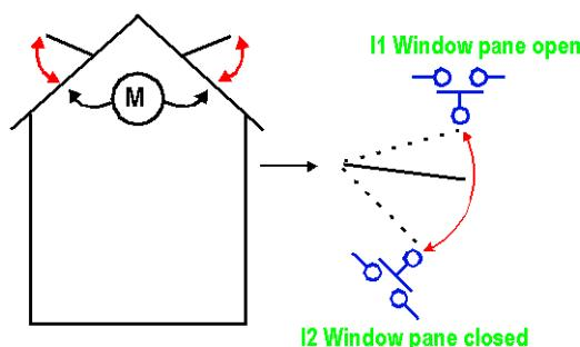
During the day, the window panes open to ventilate the structure from 12:00 to 15:00, at the time of day when, in principle, the temperature is the highest. However, if the temperature is less than 10 °C, the window panes do not open, or when they are already open, they close.
