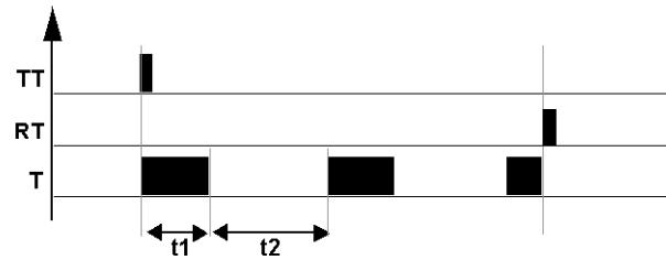
**NOTE:** Each rising edge on the TT<sub>x</sub> input resets the timer value to 0.
