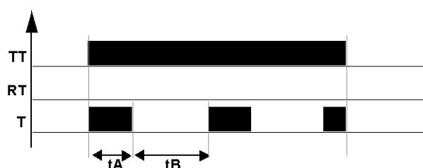
Type I is **Flasher unit; Press to start/stop**. The following diagram shows the operation of the type I timer:
