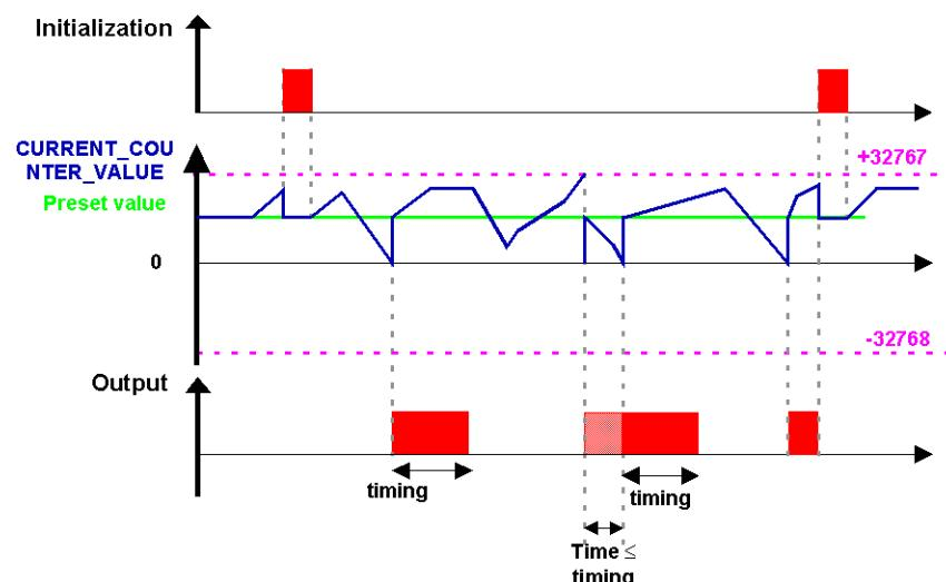
The output switches to the Inactive state when the predefined pulse duration value has run out. If the switch condition is Active before the switch to the Inactive state, the output pulse is extended by the **Duration of pulse** (Timing).
