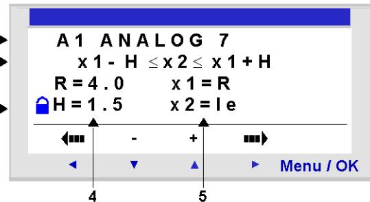
In this case: The comparison condition is verified when the power to the input terminal  $I_e$  is between 2.5 V and 5.5 V.
