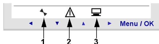
**1:** Indicates the state of the smart relay. In RUN it is in motion, in STOP it is immobile.
