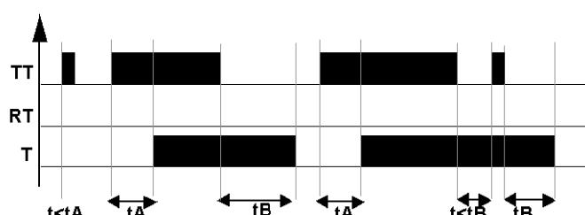
Type L is **Flasher unit, control held down asynchronously**. The following diagram shows the operation of the type L timer:
