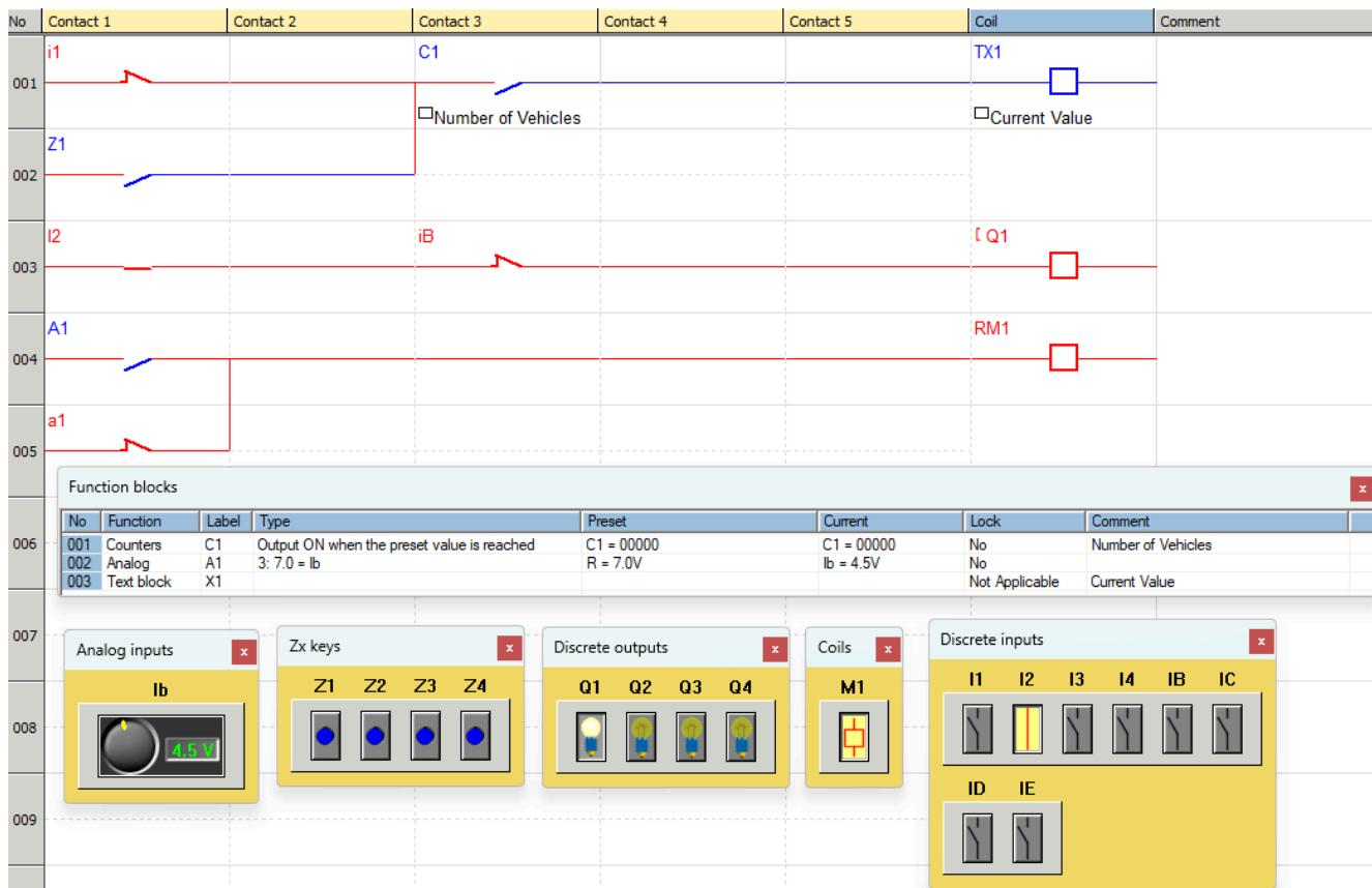
For the simulation to run, you must switch to **RUN** mode using the corresponding icon.
