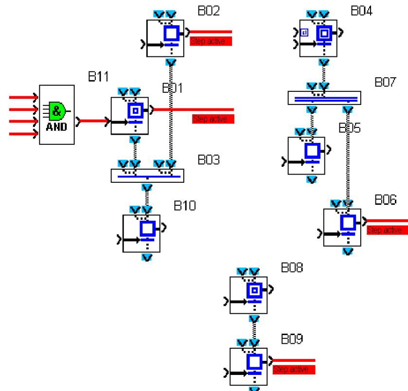
Initialization while the program is on. Initial phase 4 underway, as **Reinitialization** input of B04 block set to ON. Step B04 active in the second SFC (stable status). Steps B03 and B08 active in the other two charts are not affected.
