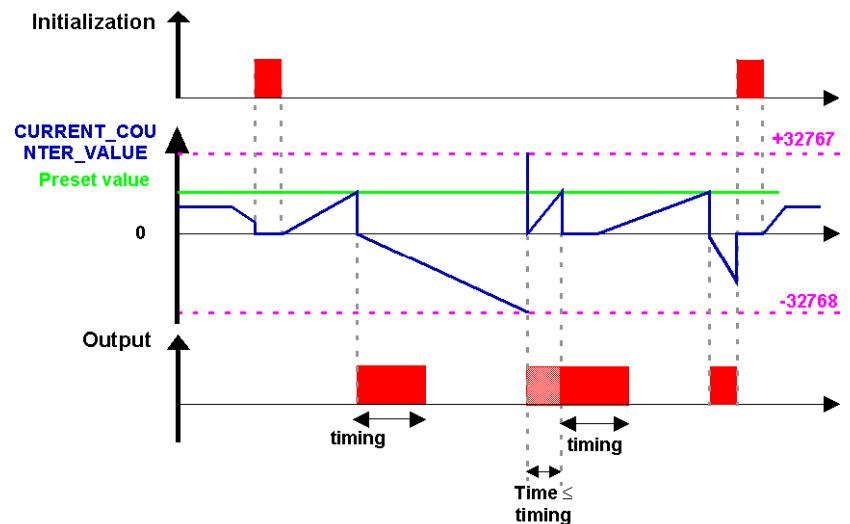
The output switches to the Inactive state when the predefined pulse duration value has run out. If the switch condition is Active before switching to the Inactive state, the output pulse is extended by the **Duration of pulse** (Timing).
