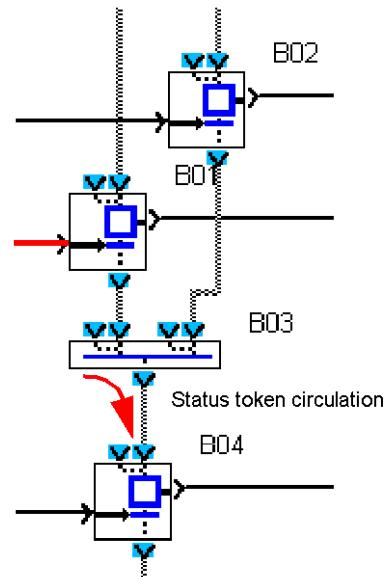
Phase 3, operation in progress: B04 step 1 active (stable status):
