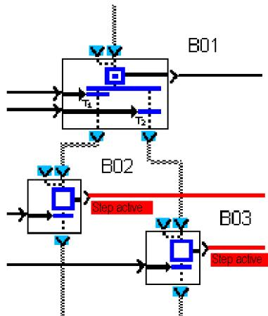
**NOTE:** If you want the choice between the two following operating phases to be exclusive, one of the two transitions must be commanded by an **AND** combining the command of the first transition with the reverse of the second transition command.
