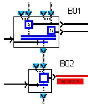
If a single token is present in one of the upstream steps and the other is empty (inactive), then even if the transition is set to ON, nothing happens. The step containing the token stays active (Discrete observation output of the step set to ON) and the downstream step (B03) stays inactive.
