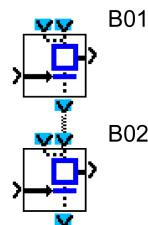
To show the fact that the switching off of operating phase B01 is followed (in sequence) by operating phase B02, the B01 status token circulation output is linked to one of the circulation inputs of the B02 status tokens.
