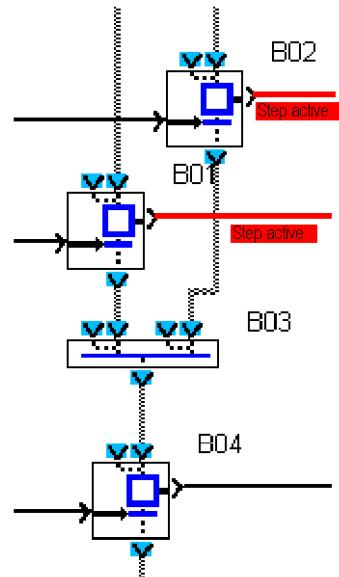
Simultaneous end of operating phases 1 and 2: transition B01 and B02 simultaneously active (momentary status):
