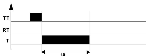
Type D is **Symmetrical flashing** for control held down synchronously. The following diagram shows the operation of the type D timer:
