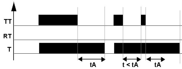
Type B is **On pulse one shot** for a pulse calibrated on the command input rising edge. The following diagram shows the operation of the type B timer:
