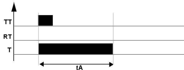
Type W is **Timing after pulse** for a pulse calibrated on the command input falling edge. The following diagram shows the operation of the type W timer:
