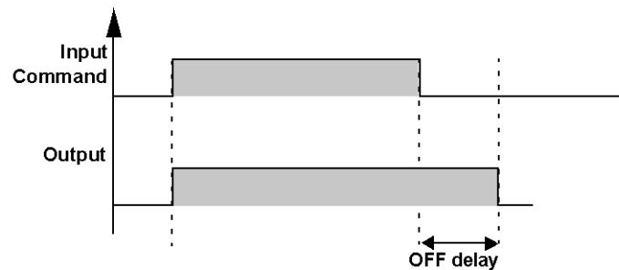
**NOTE:** Each pulse on the **Command** input of the Timer block resets the present value to 0.
