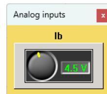
The analog value can be modified by adjusting the potentiometer (click).
