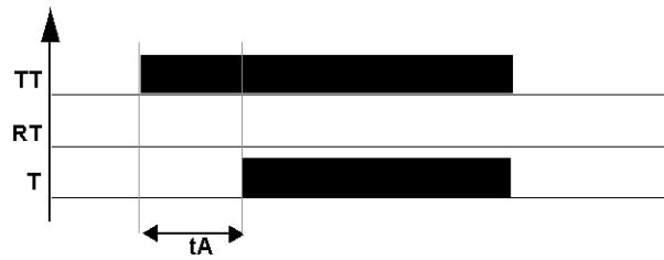
Type a is **Active, Press to start/stop**. The following diagram shows the operation of the type a timer:
