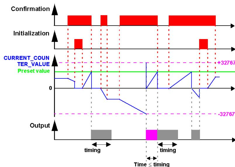
The output switches to the **Inactive** state when the predefined pulse duration value has elapsed. If the switch condition is Active before the switch to the Inactive state, the output pulse is extended by the **Duration of pulse (Timing)**.
