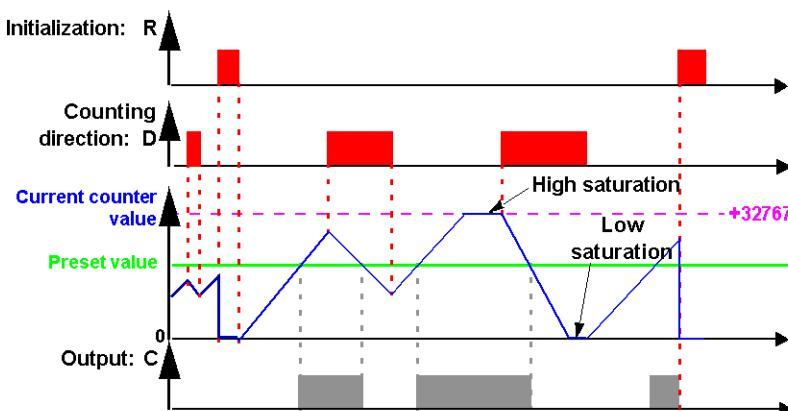
The following figure shows the operation of the counter when downcounting (**FROM**) from the preset value:
