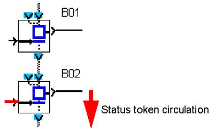
If step 1 is not active, the associated operating phase (B01) is not in progress, and by definition, the status token is not present in step 1. Therefore, turning ON the Discrete input of transition command 1 that authorizes the transition will have no effect as there is no token in step 1 (the token cannot be passed on).
