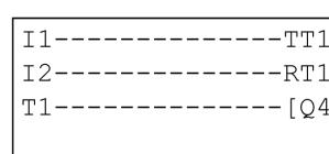
To obtain the desired operation, you should use a type B timer (On pulse one shot), and configure the duration of the timer for 2 minutes 30 seconds. To thus
