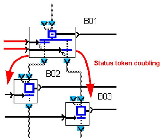
Operating phase 2 and 3 in progress: steps B02 and B03 active (stable statuses):
