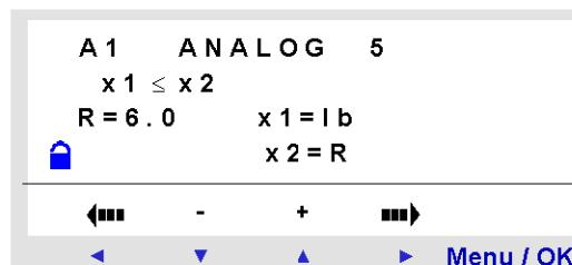
The comparison operator 5 is chosen, that is “inferior or equal to”.
