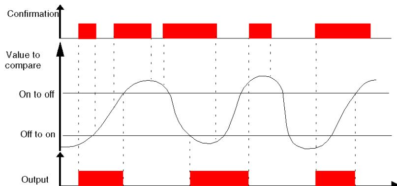
The figure shows the possible output states when the **Off to on setpoint** is higher than the **On to off setpoint**:
