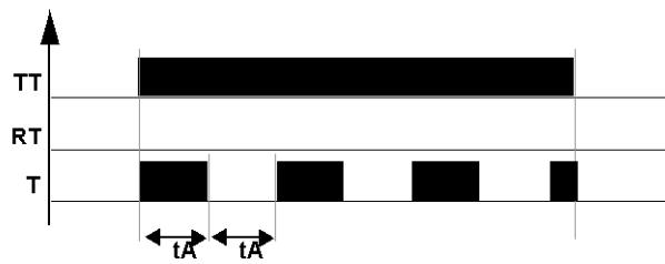
Type PD is **Symmetrical flashing, Start/stop on pulse**. The following diagram shows the operation of the type PD timer:
