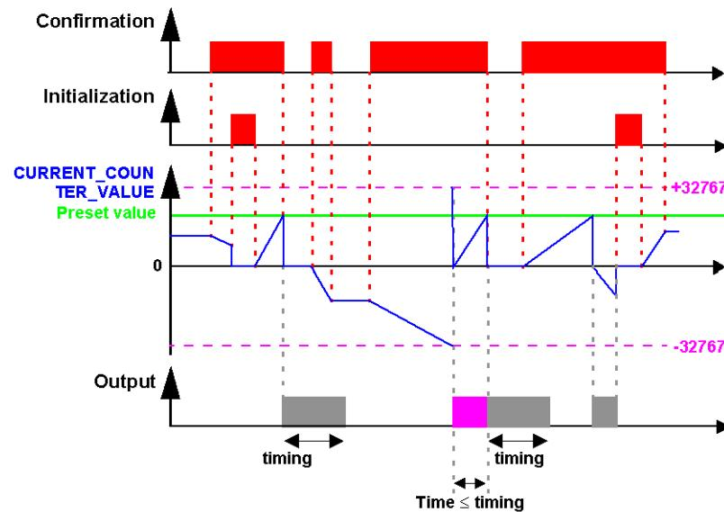
The output switches to the **Inactive** state when the predefined pulse duration value has run out. If the switch condition is Active before the switch to the Inactive state, the output pulse is extended by the **Duration of pulse** (Timing).
