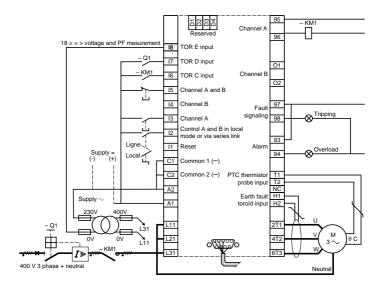
The LT6 can be connected to a multi-drop bus using standard RS 485 or an RS 232 link
