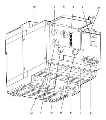
1 and 2 Rotary selectors for setting the rated motor current
