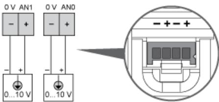
The (-) poles are connected internally.
