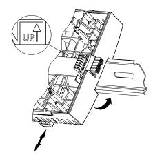
**NOTE:** Install the terminal base on a horizontal DIN rail. This position provides proper cooling air flow through the electronics module.
