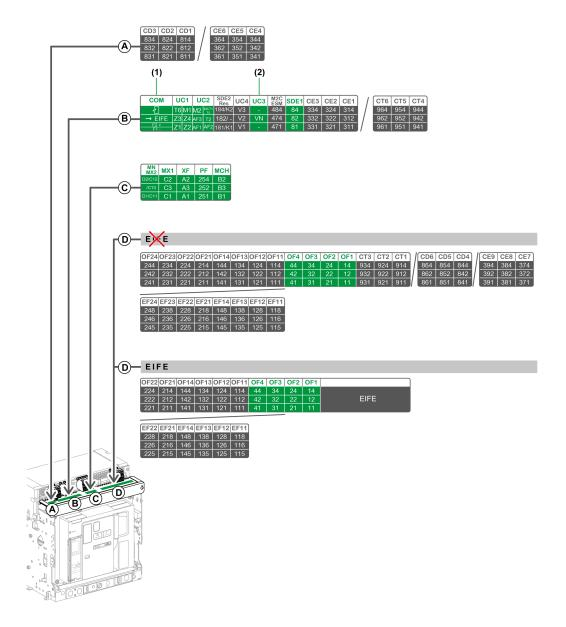
Terminal block supplied as standard on the chassis
