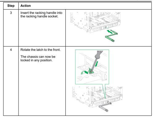
**NOTE:** To return the chassis to locking only in the disconnected position, rotate the latch to its original position at the rear.
