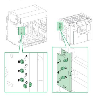
The pin combination selected on the chassis must correspond to the pin combination selected on the device (see following table). For example, the combination ABCD on the chassis corresponds to the combination 567 on the device.
