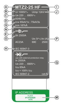
J Uimp: rated impulse withstand voltage
