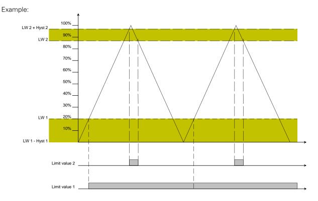
The limit values and the hysteresis characteristics are specified as a percentage of the full measuring range. When setting the limit values and the pertaining hysteresis, a safety margin of about 1% from the minimum value (0%) and from the maximum value (100%) should be observed. Or else the signals cannot underrun or exceed the respective thresholds. In this case, the limit-value object can transmit at maximum one telegram as shown for limit value 1.
