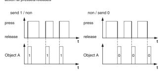
Object A = 1 Bit action at pressed/released
