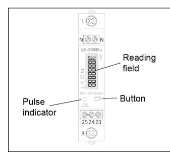
**Reading field** – LCD digital indicator displaying the value of the measured parameter.
