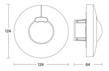
Possible mounting height: 2,00 m – 4,00 m Orange: radial and tangential
