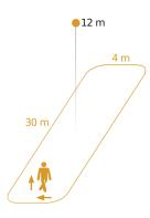
Possible mounting height: 4,00 m - 16,00 m Orange: radial and tangential
