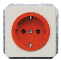
DELTA profil, titanium white SCHUKO socket outlet 10/16 A 250 V Orange bezel (ZSV) With screwless Connection terminals Cover plate 65x 65 mm
