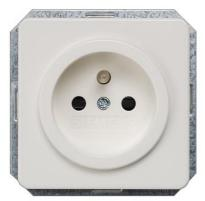
DELTA profil, titanium white Socket outlet 10/16A 250 V with grounding pin with increased touch protection 2-pole according to CEE7, with Cage clamp terminals Cover plate  $65x\ 65\ mm$
