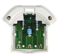
DELTA programs Overvoltage protection module as replacement, for SCHUKO socket outlets with overvoltage protection
