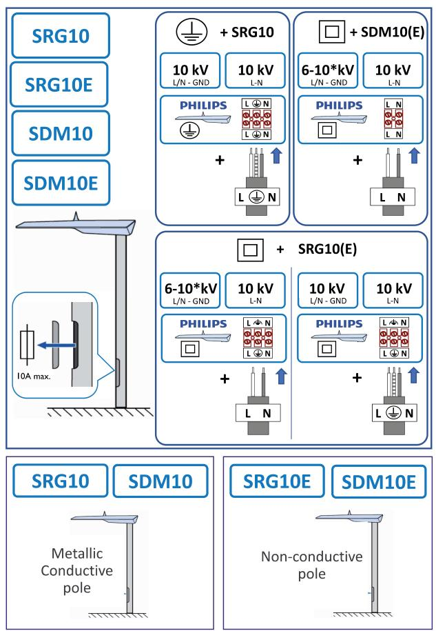
\* 10kV for L/N – GND non-conductive connection
