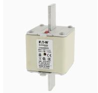
**Fuse-link, high speed, 1100 A, AC 690 V, DIN 3, aR, DIN, IEC, dual indicator, live gripping lugs**
