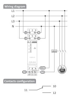
Changeover contact of the relay allows to connect a visual or audible signalling system that informs about the relay activation, which means switching off the motor.
