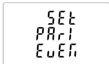
From the set up menu, use **P▼** and **MD/PF/HZ▲** buttons to select the parity option.
