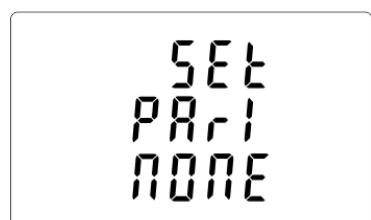
Use **P▼** and **MD/PF/HZ▲** buttons to choose parity EVEN/ODD/NONE (default).
