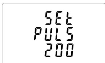
From the setup menu, use **P** and **MD/PF/HZ** buttons to select the pulse width option.
