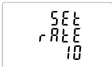
From the setup menu, use **P** and **MD/PF/HZ** buttons to select the pulse rate option.
