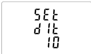
From the setup menu, use **P ▼** and **MD/HZ ▲** buttons, to select the DIT option.
