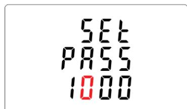
Use **P ▼** and **MD/PF/HZ ▲** buttons to set the first digit and press **E ▶** to confirm your selection. The next digit will flash.
