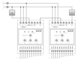
According to the above scheme, any number of controllers can be combined.
