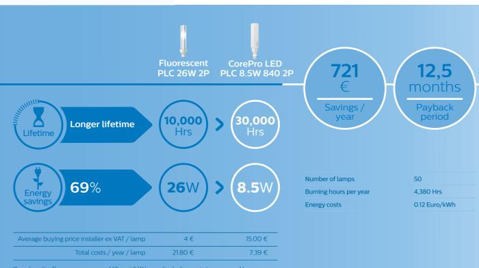
Based on the European average of 12 cent/kW hours (including maintenance and lamp replacement cost)
