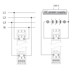
Direct measurement of 3-phase network voltage Direct voltage measurement DC circuit
