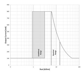
$$I_{\text{OUT[A]}} = \frac{5V}{R_{\text{set}[\Omega]}} \times 1000$$
