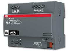
For controlling blower convectors. Supports 2-pipe and 4-pipe system for heating and cooling. The fan speed levels can be switched using a changeover or step switch function. Three contacts for switching a three-stage fan. Two contacts for activating the heating and cooling valves. Supports 24V and 230V valves. With two binary inputs for connecting dewpoint and condensation contacts. The scanning voltage is provided by the device. The bus connection is provided via the enclosed bus terminal.
